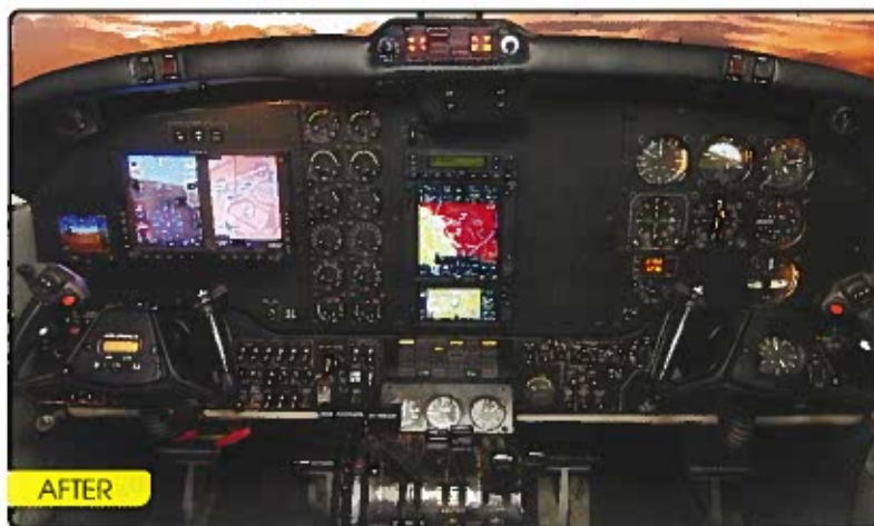
A more-reliable, solid-state glass cockpit was installed for better situational awareness, reliability and minimized downtime.
